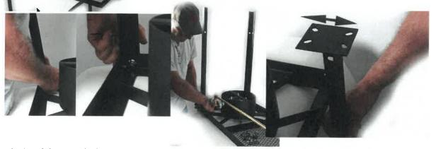
4: Attach legs snugly, but DO NOT tighten the screws all the way. You will need to stand the burner, right side up later, to be sure it is level, and only then will you tighten all the screws. Once legs are attached, 5: Install the Bottom Grate and Wheels as shown below. The bottom grate attaches to the inside of each leg.
