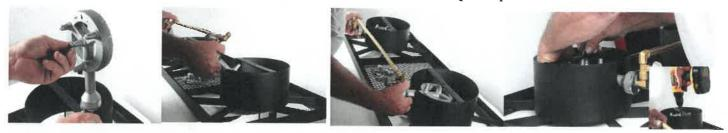
3: Remove mounting screw from bottom of both burners, place top plate of stove on a flat surface. Then place burners and valve assembly in place, and tighten mounting screws securely with a 3/8 socket.
