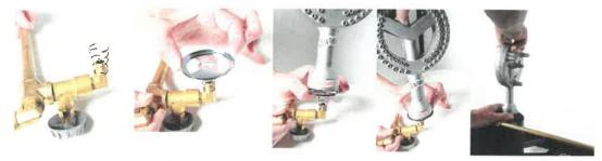
Piece together valve assembly—— 1: Place spring small side touching brass. 2: Place shutter plate on bottom of burner as shown above, and turn to screw burner onto brass valve. Repeat steps for both burners.
